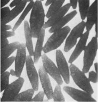
Fig. 11. Effect of V_1/V_f ratio on the shape of acrylic fibers spun from a rectangular hole with an aspect ratio of 9.8.
